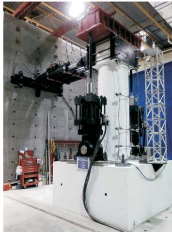
Figure 2: Experimental setup: as-built setup and specimen.
